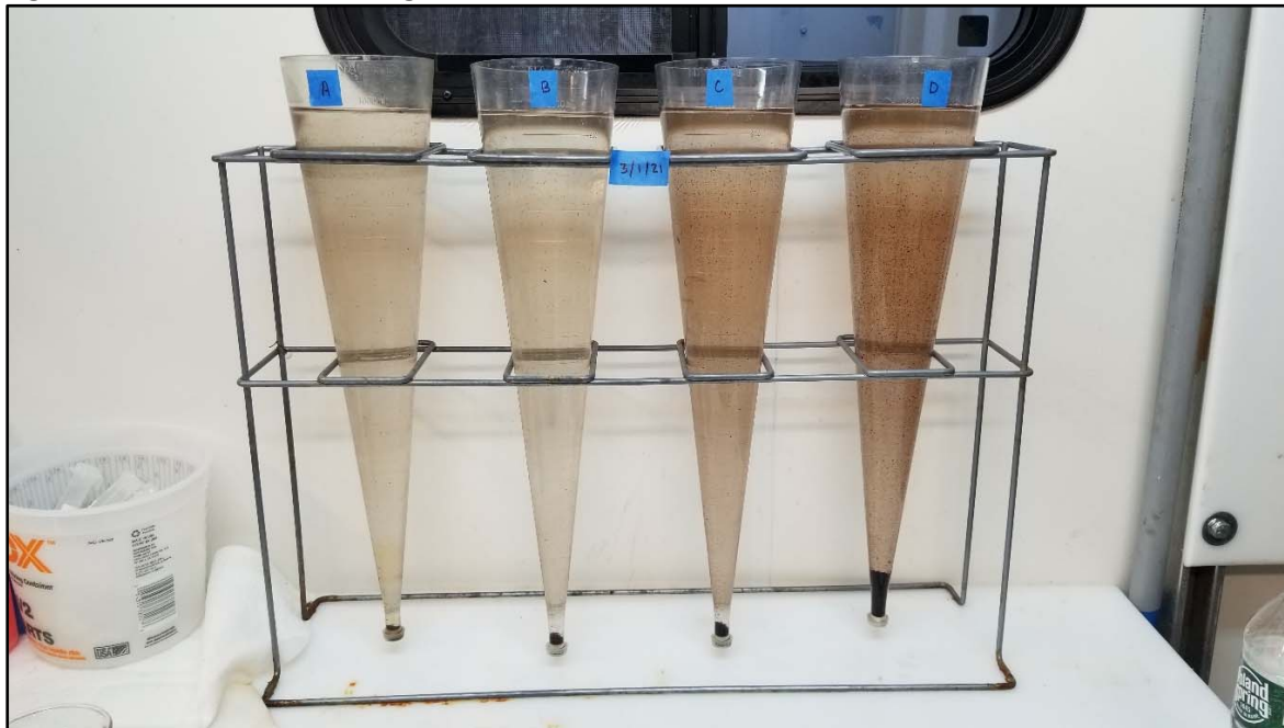
Figure 4.08: Backwash Settling in Imhoff Cones for Well 2 – Trial 4
