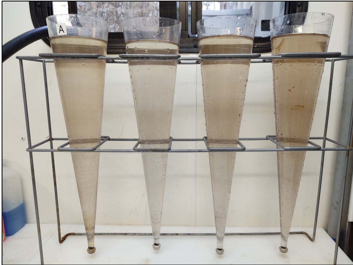
Figure 4.07: Backwash Settling in Imhoff Cones for Well 5 – Trial 2
